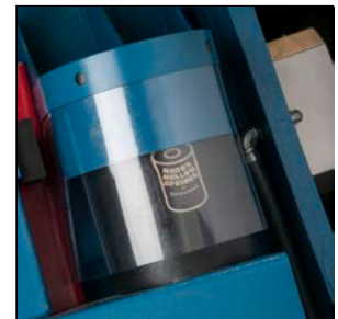
SmoothCoil™ suspension minimizes transmission of unwanted vibration
